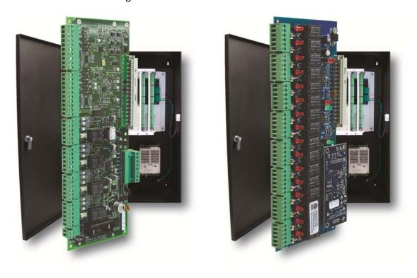
They come in a variety of Access Controllers, Input, Output, or Intercom controllers. Each controller has its own CPU and operates on an Echelon Communications Network.
